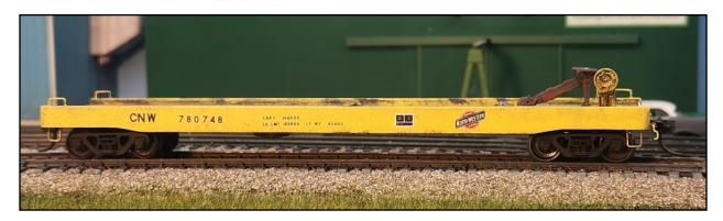
CNW 780748 and SOU 15040 are heavily modified Front Range kits for a Southern Railway prototype. Both cars had wire grabs and cut levers added, were lowered and weighted. Cars were painted, decaled and weathered with acrylic craft paint. *Fritz Dahlin, Chesapeake Division*
