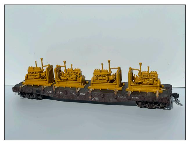
The model is a modified Athearn kit shortened from 50' down to 44'-6" to match a Santa Fe class Ft-M car. The underside was completely rebuilt, including a Type K brake system with all pipes and rods. The generators are from Life Like and the blocking was cut from Evergreen styrene. *Ken Wilson*
