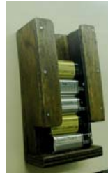
Figure 4 shows two finished throttle pockets. I suggest gluing a small piece of foam rubber to the inside bottom of the throttle pocket where the bottom of the throttle will rest.
