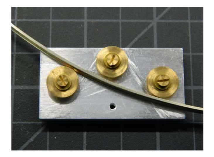
**Roller bearings** Aluminum back plate Code 70-100 rail Final adjustment using finger pressure and compass-drawn template
