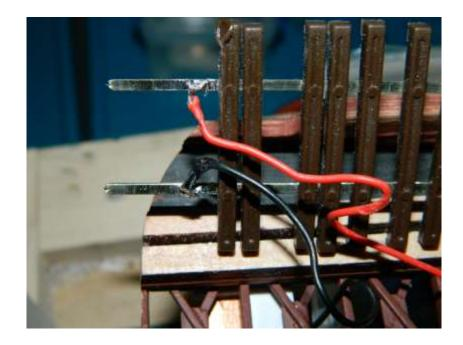
Wires soldered to lugs on disk, then attached to rail bottom at both ends of the bridge (disk)
