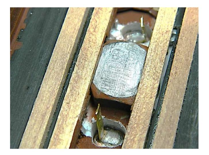
Bolt epoxyded to styrene plate
