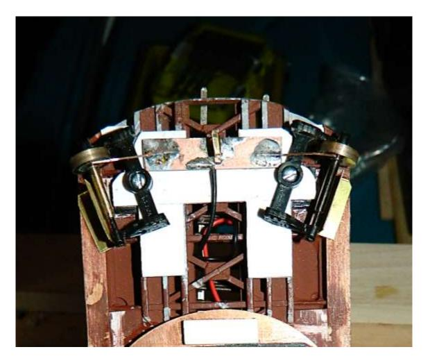
Support framework of styrene sheet attached to bridge bottom
