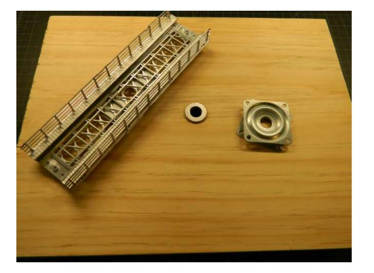
This is my test bed – piece of pine with a hole for a 0.5" diameter brass tube sleeve bearing and washer end into which a 12mm M12 fits nicely
