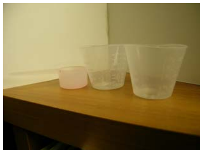
Measure and mix the RTV - New Method by volume vs by weight. Either way 1:10
