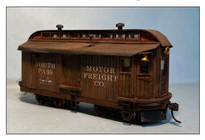
This is my latest project. I finished it in my quest for the Master Builder-Motive Power certificate. It is a Conowingo Models "Boxbug Doodlebug" kit that I modified in several ways, including installation of Stanton power wheelsets instead of a Bachmann 44-ton switcher power chassis. I also added a front coupler and a plow/cowcatcher
