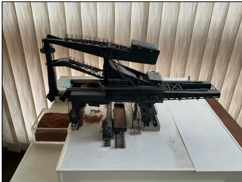
Left: Contest model of superdetailed Walthers Hulett. Ten motors crab, trolley, leg down, open bucket in ship's hold, lift bucket, trolley, discharge ore into ore bin and Larry car, shuttle Larry car and discharge ore to gondola, en route to blast furnace. First place, kit class, NMRA National Convention, Milwaukee, Wisconsin, 2010.
