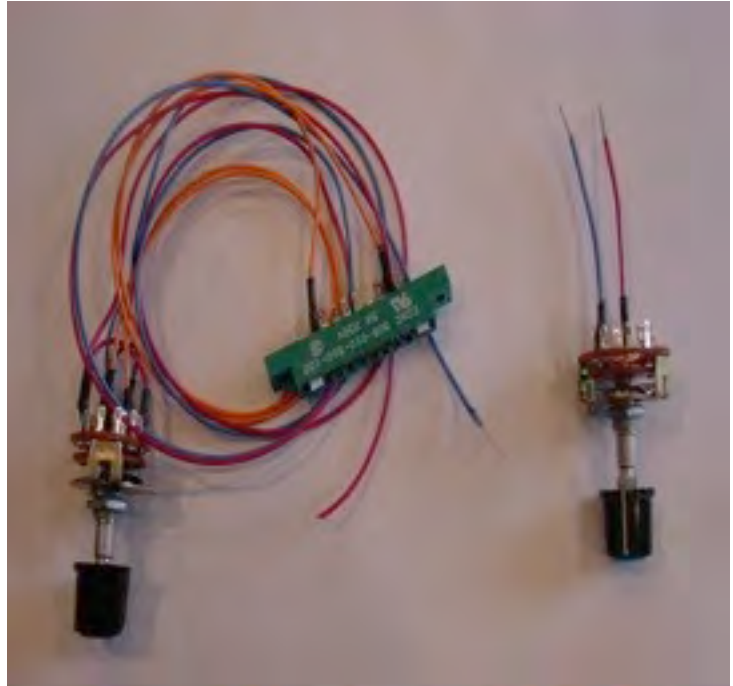
Pete pre-wires the rotary switches and connector at the workbench - MUCH easier than working under the layout!
