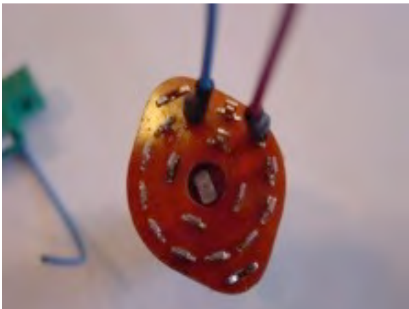
The back of the rotary switch is pre-wired.
