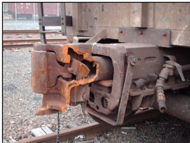
Photo right: A broken coupler on Amtrak rolling stock.
