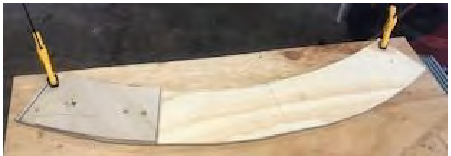
Marking a helix segment using a pattern that had twenty four inch inside radius, 26 inch track radius, and 28 inch outside radius
