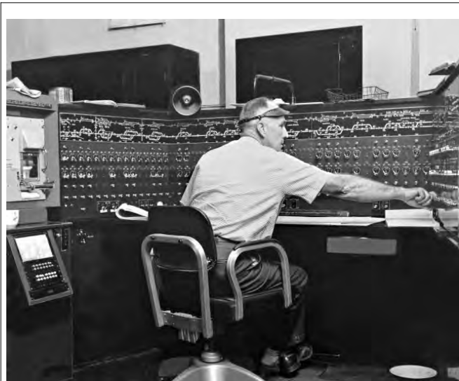
A Dispatcher is operating a CTC panel. There is a railroad diagram at the top of the panel. Lower on the panel are toggles for the dispatcher to remotely operate turnouts along the route.
