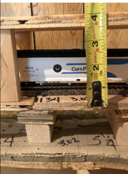
Using a hopper car to verify the clearance between level 1 and level 2 is sufficient
