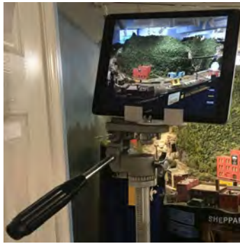
A 3D printed iPad holder for a tripod allowed for an iPad to serve as another camera.
