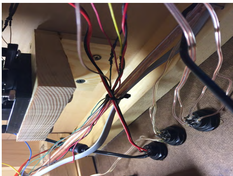
Figure 5 - Mounting Bracket with RTM and Tortoise Switch Machine Attached to Underside of Layout
