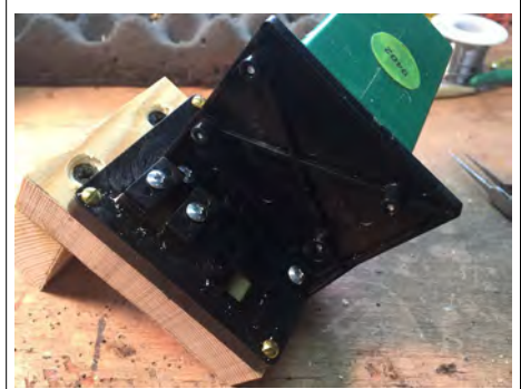
Figure 4 - RTM with Tortoise Switch Machine Attached to Mounting Bracket
