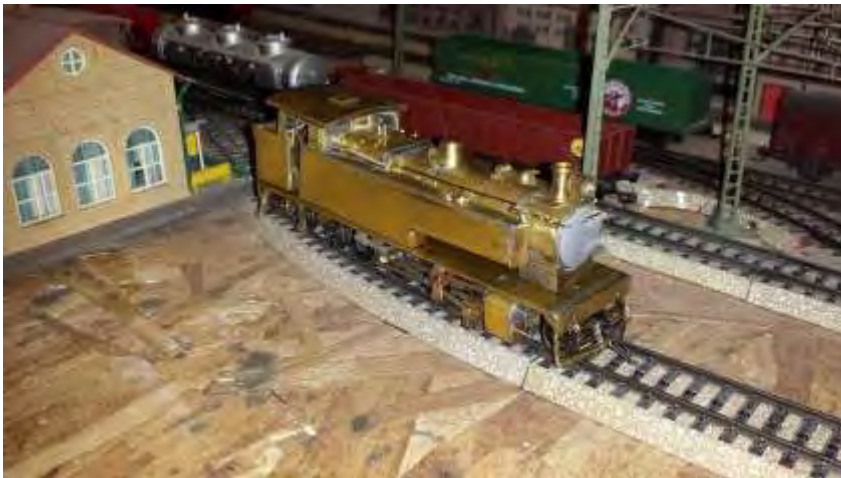
The smokebox door of this Kistons model was printed using ABS
