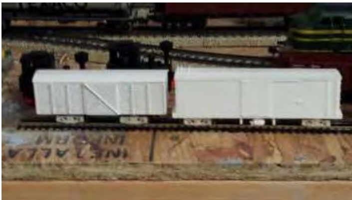
On the left, a narrow gauge box car. The body and roof are made from PLA. The trucks, ABS. On the right is a F&C commercial model with the same ABS printed trucks.
