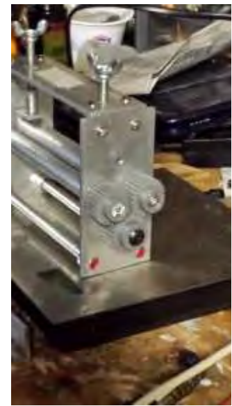
An example of parts for home built tools: the cogwheels in this metal sheet roller were 3D printed in ABS.
