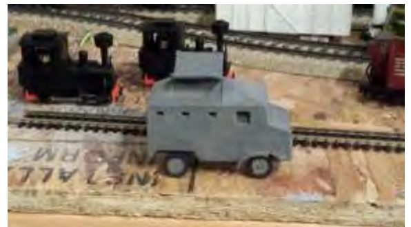
A "Butterfly" type armored vehicle printed entirely in ABS. The wheels were printed separately to reduce the need for supports and rafts. No smoothing of the surface was applied.
