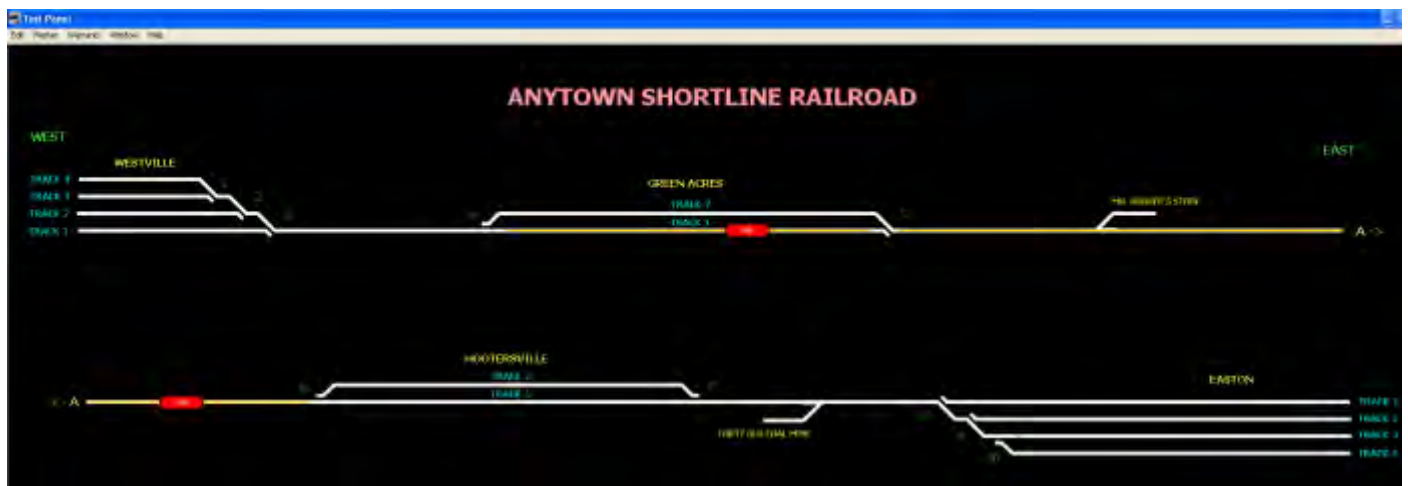
Fig. 16 As both trains progress across the railroad they trip occupancy detectors in each area they are present. As they leave an occupancy block it returns to the color white stating the block is clear. Note that Train 17W is in sensor block LS30 which is yellow on both the upper and lower rows in the panel diagram.
