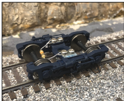
Figure 3: Looking at the top of the truck with the resistor leads trimmed, screwed in place and bent downward toward the track to keep the resistor from rubbing against the underframe or wheels. (Left)
