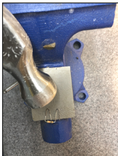
Figure 2: After the leads were formed, I flattened them with a hammer on the anvil part of my vise. (Left)
