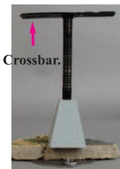
The O27 trolley track is supported by 4" crossbars from Texas Lamp Parts. See photograph on next page. Threaded lamp pipe screws into the crossbar. At the bottom the pipe is supported by wood simulated concrete bases which supply some support. The pipes are securely fastened by washers and nuts.
